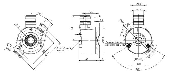
CHO5\_14 connection S5R (radial cable), DAC 9445/015\* mounted on the cover
