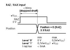
Note: Do not connect other pinouts, connect DIRECTION and RAZ to a potential (RAZ at 0V if not used).
